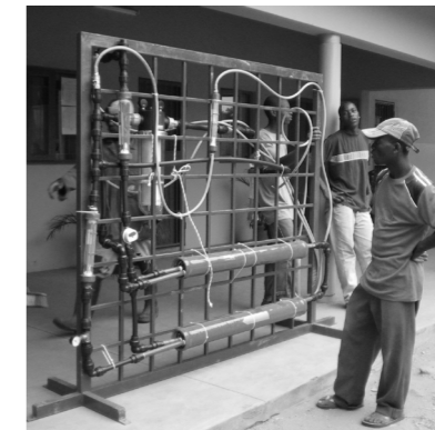
Jornadas formativas y planta potabilizadoras instaladas por AQUAPOT en Ecuador y Mozambique Learning sessions and potabilization units set up by AQUAPOT in Ecuador and Mozambique
