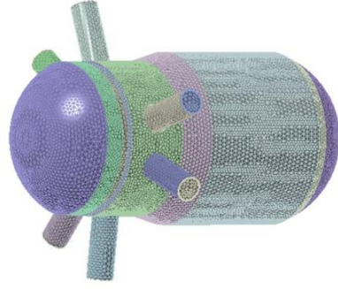
FIG. 4_9. Malla no estructurada vasija reactor PWR simulado con Ansys CFX ® Unstructured mesh of the vessel PWR reactor simulated with Ansys CFX ®
